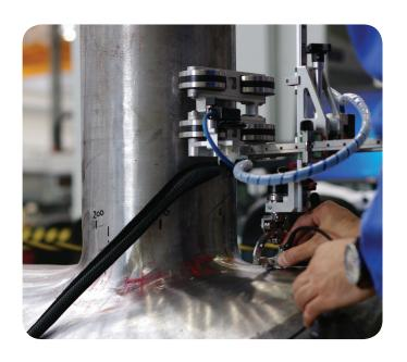
NozzleScan is a versatile manual scanning solution developed for the inspection of nozzle welds in both set-through and set-on configurations.
